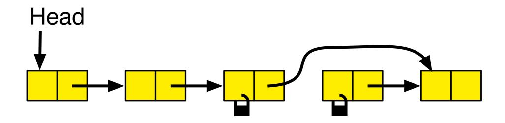
Remove locked node by a pointer swing
